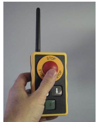
Emergency Stop-Remote Control Panel
