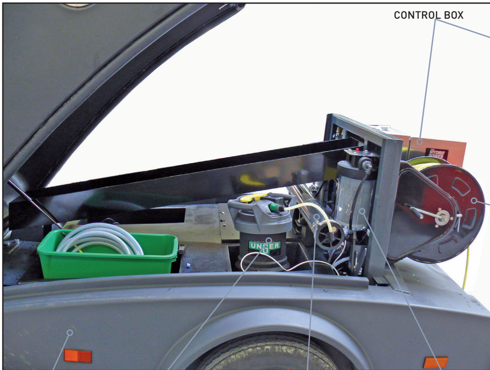
WATER TANK ION EXCHANGE RESIN FILTER (DI) HydroPower DI (DI24T) REVERSE OSMOSIS FILTER (RO) CARBON PRE-FILTER CONTROL BOX
