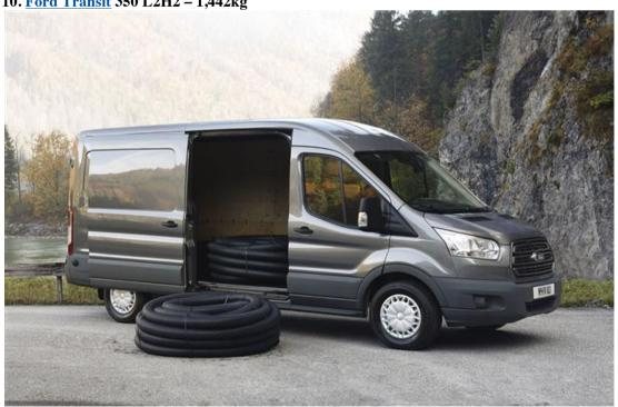
Despite being the most popular commercial vehicle in the UK, the new Ford Transit offers less payload than all of the other 3.5 tonners. The latest model, which was introduced in 2014, is a lot larger than most of the competitors (load volumes start at 9.6 cubic metres), and this added weight pushes the payload to under 1.5 tonnes.
