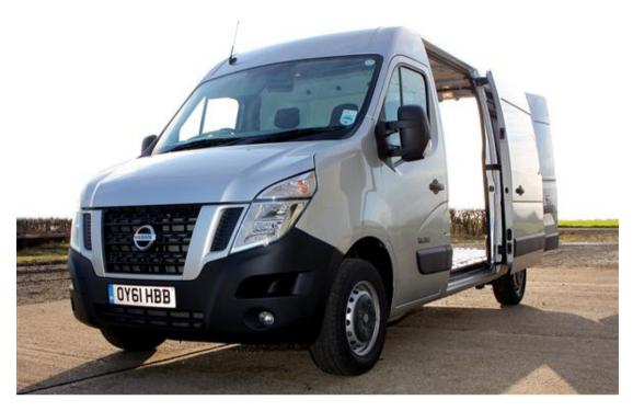
Although the Nissan NV400 is essentially the same van as the Vauxhall Movano and Renault Master, it is over 60kg heavier due to the redesigned and distinctive front grille, bumper, lights and bonnet. At 1,620kg, it still overs a respectable payload.
