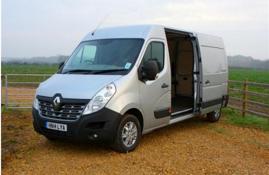
At the top of the list are the Vauxhall Movano and Renault Master. While they lack the refinement and some of the safety systems of newer competition, these Vauxhall Movano and Renault Master weigh a little over 1,700kg, which means they boast a class-leading payload of 1,684kg.
