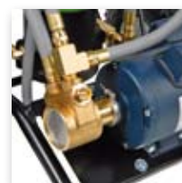
Pump relief safety valve
