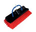
For easy and thorough solar panel cleansing from various application angles. Compatible to telescopic HYBRIDPOLE and telescopic CARBONPOLE in connection with adapter QLEEN to LEWI or aluminium pivot joint (page 6). Bristle thickness 0.35 mm, bristle length 40 mm, fanned.
